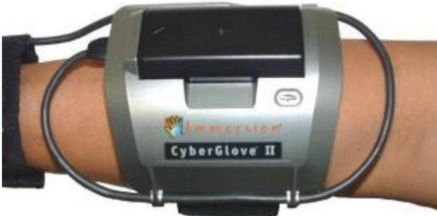
The interface module can be mounted in either direction to accommodate various arm lengths.
