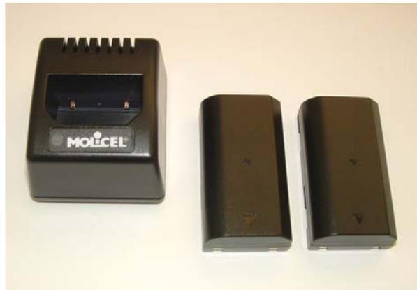
Before you can use your CyberGlove system you will need to fully charge one of the two batteries provided. Please note the proper charging and safety precautions below. While the battery is charging, which takes about five hours, proceed with installation of the IOGEAR adapter and software.
